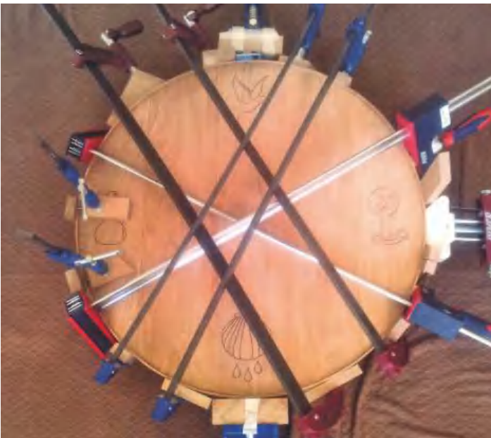
▲ Pic.17 I needed to use a large number and variety of clamps to make sure the lath would be correctly glued into position
